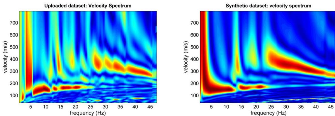
**Figure 3.** Rayleigh waves (radial component - RVF): on the left the field data, on the right the synthetics of the retrieved model (reported in Figure 5).
