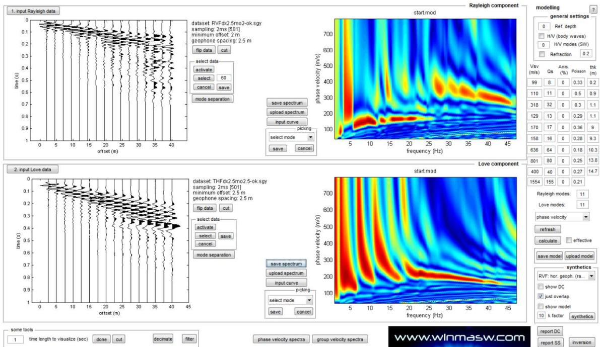
**Figure 2.** Field data. *Upper panel:* Rayleigh waves (radial component - RVF); *lower panel:* Love waves (THF).
