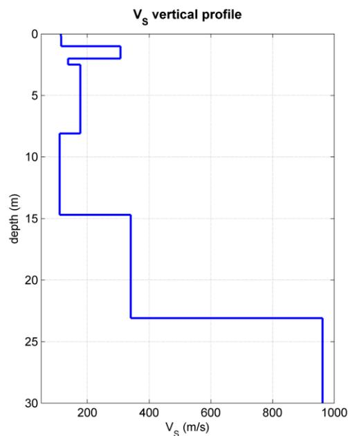
**Figure 5.** Identified  $V_S$  model.
