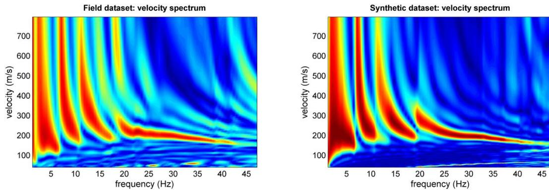
**Figure 4.** Love waves (THF component): on the left the field data, on the right the synthetics of the retrieved model (reported in Figure 5).
