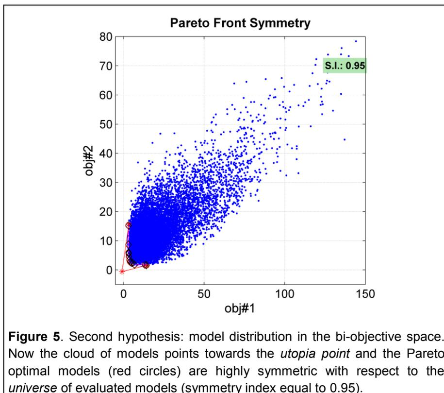
**Figure 5.** Second hypothesis: model distribution in the bi-objective space. Now the cloud of models points towards the *utopia point* and the Pareto optimal models (red circles) are highly symmetric with respect to the *universe* of evaluated models (symmetry index equal to 0.95).
