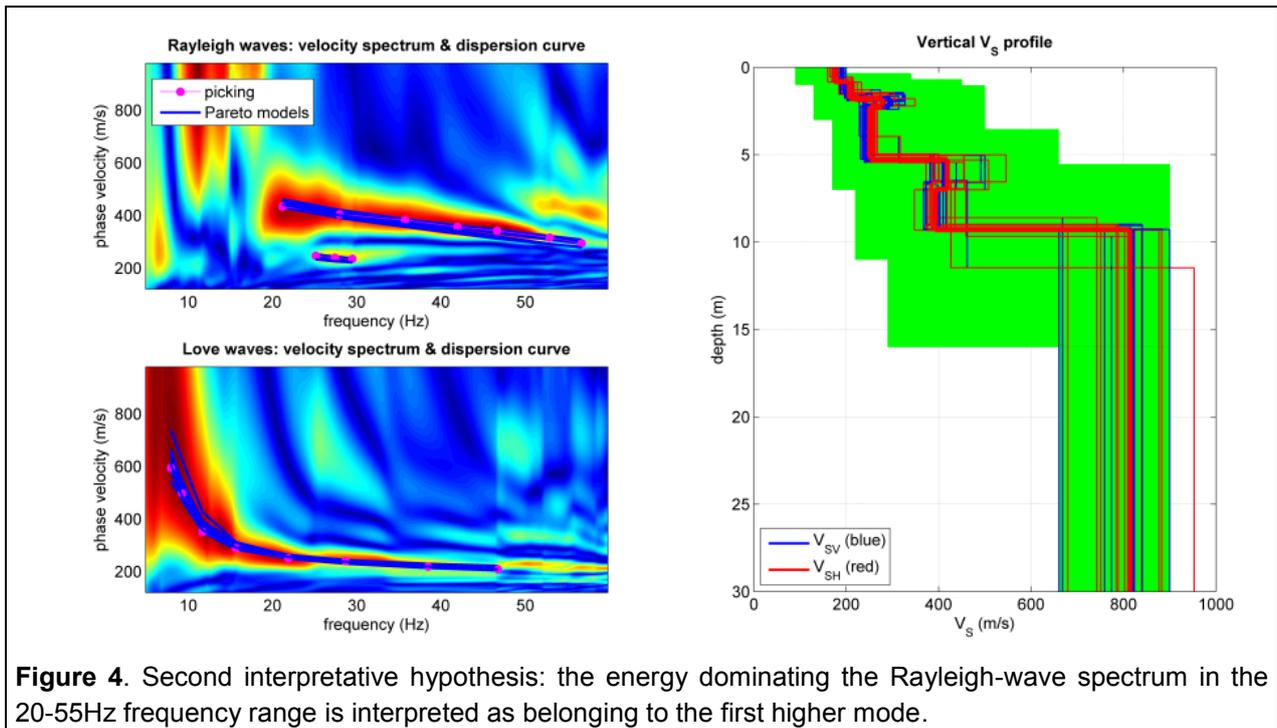
**Figure 4.** Second interpretative hypothesis: the energy dominating the Rayleigh-wave spectrum in the 20-55Hz frequency range is interpreted as belonging to the first higher mode.
