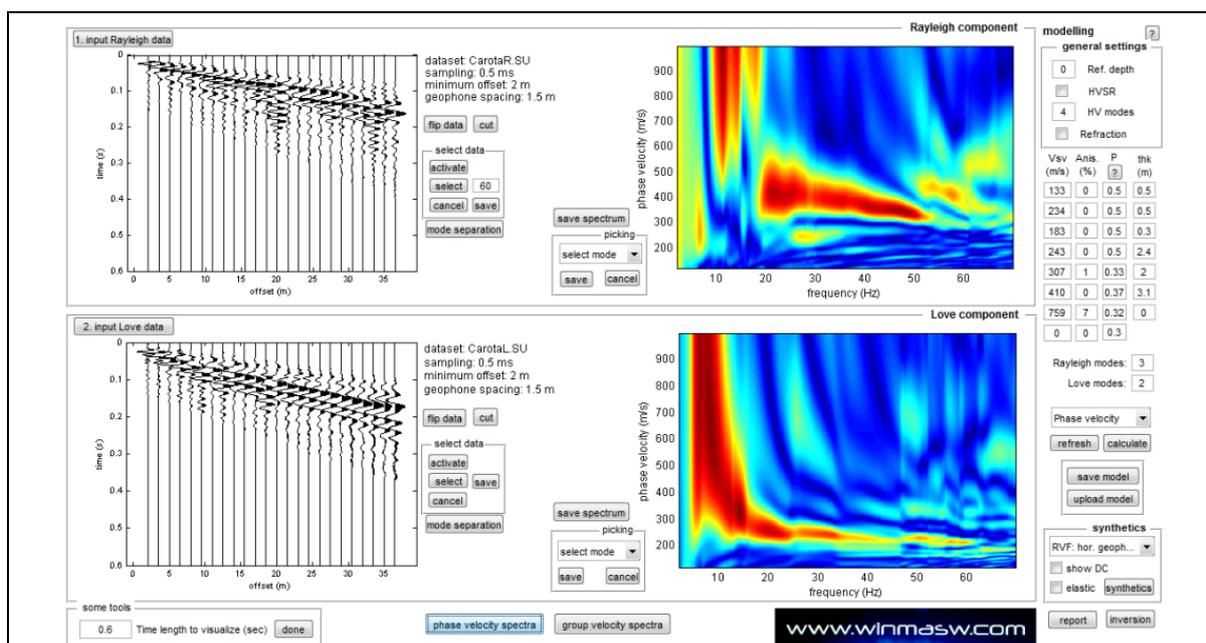
**Figure 1.** Upper panel: Rayleigh waves (RVF component); lower panel: Love waves (THF).
