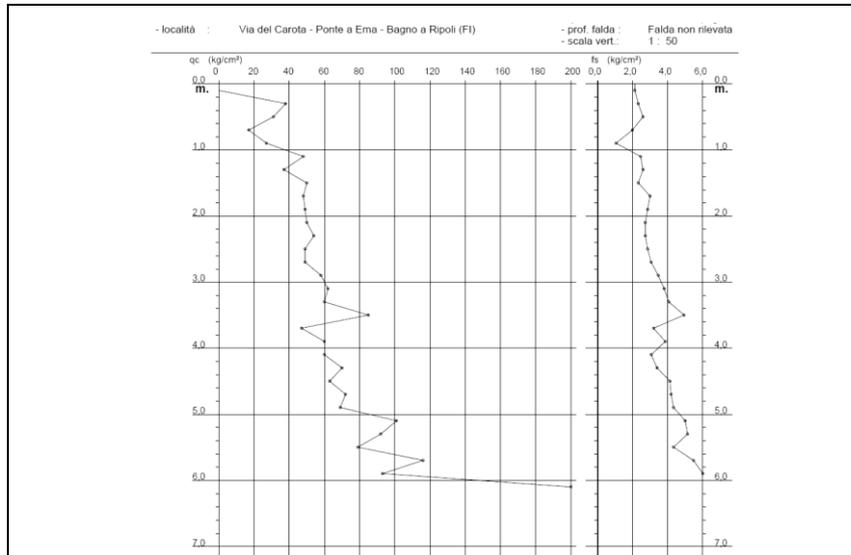
**Figure 6.** Cone Penetration Test: at a depth of about 6 meters CPT stopped because of a stiff layer. Compare with the horizon put in evidence by the joint analysis presented in Figure 4.
