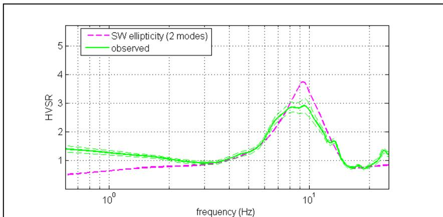
**Figure 7.** Observed and modeled (average model from the Pareto front models obtained from the second interpretative hypothesis) *Horizontal-to-Vertical Spectral Ratio* (from microtremors).
