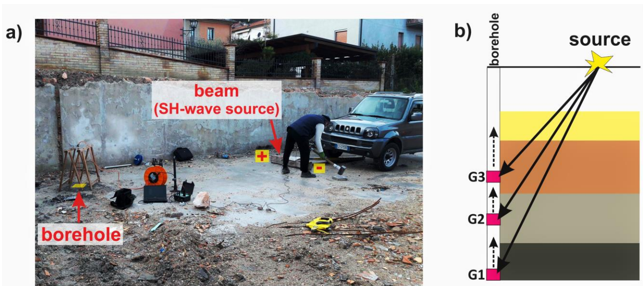
Figure 4. Field operation: a) downhole survey for the generation and acquisition of SH waves. The wooden beam is secured/coupled to the ground thanks to the weight of the car (this way it transmits most of the energy generated by the hammer impact). The survey took place in San Severino Marche (IT) after the 2016 central Italy seismic crisis. Courtesy ABgeo ( www.abgeo.org ). Data processing: a) several software applications for the processing of DH data assume a linear path but this does not represent a correct solution (see Figure 5).
